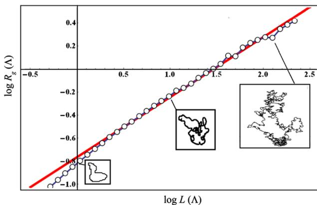
FIG. 3 (color online). A Log-log plot of the radius of gyration  $R_g$  against loop length,  $L$ . For illustrative purposes, three loops of different lengths are shown. The red line is a fit to the straight line section (0.2–2.0) on the  $\log L$  scale and has a gradient of 0.52. Links between two loops were only found for  $\log(L) > 0.2$ .
