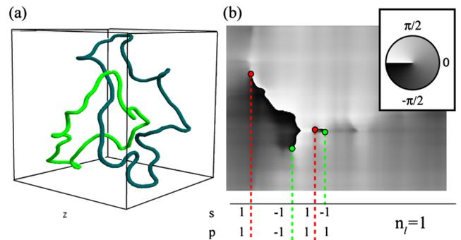
FIG. 2 (color online). Linked vortex loops. (a) Shows a linked pair of vortex loops,  $\mathbf{a}$ ,  $\mathbf{b}$  in a simulated speckle field. (b) Shows the chord angle  $\theta_{\mathbf{a},\mathbf{b}}(i,j)$  pairs of points on the loops projected into viewing plane. The singularities in the chord angle correspond to signed crossings with values  $s$  and  $p$  given in the table.
